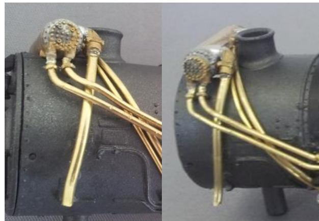
A slot was cut in the top of the smokebox to take the Feedwater heater using a razor saw (laterally) and drilled with an electric mini drill to make the ends of the slot. This results in a rectangular hole which disappears when the heater is placed in it. The rather thick brass wire was carefully bent as required, positioned with eyebolts, and superglued in position. This needs to be taken to the full lengths as required and connected at both ends.
