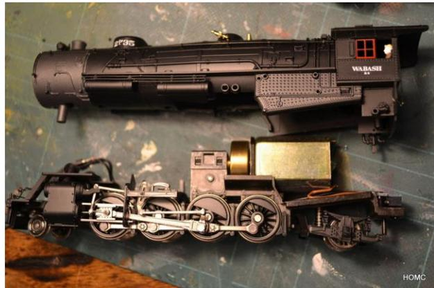
The approach of this modification was to give the impression of an M3s or M3as and the photos show that this is achieved without attention to minute detail. One main compromise is with check valves, which have been simulated with inverted stanchions where simulated at all. Other compromises are described at the end.
