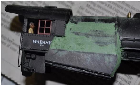
Green putty and White putty were then used to fill the gaps (above left) and give a smooth surface and this was finished with a thin sheet of plastic-card glued over the top. For this use superglue and ensure that there are no air-gaps. Other details such as boiler bands may also be added in plastic-card and MEK solvent was used for this.
